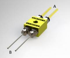
LA-MAN-2-X 2-ZONE TUBE ADAPTOR MANIFOLD (Use to join Stainless Steel Tube to Stainless Steel Tube or PU Tube) X=1 A=SS1.6mm B=SS1.6mm X=2 A=SS1.6mm B=SS2.0mm X=3 A=SS1.6mm B=PU4.0mm X=4 A=SS2.0mm B=SS2.0mm
