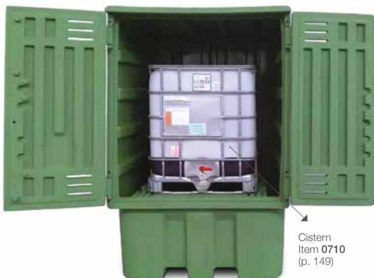
Container for 1000 lt. cistern in single-body ecological polyethylene with seamless collection tank. 180° opening doors with padlockable lever closure and internal document holder in the left door. Complete with 4 ventilation grilles to avoid gas accumulation and independent support table. Forkable. Resistant to acids (\*), bases and oils. Sump collection capacity lt. 1100.
