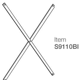
**STIFFENING CROSSPIECE** in plasticised steel plate with holes  $\emptyset$  mm. 9 and equipped with supplied with flanged nut. **To be used, in the absence of wall fixings, in the initial and final span and 1 every 3 central spans.**
