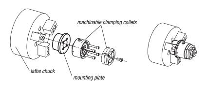
Mounting plate for holding the collet in a lathe chuck
