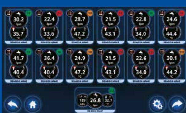
The main screen will show all circuits with information about flow and temperature. The main inlet and outlet will also show including pressure.
