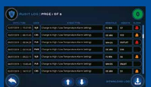
The system is equipped with Audit Log to keep track of all events including user ID tracer.
